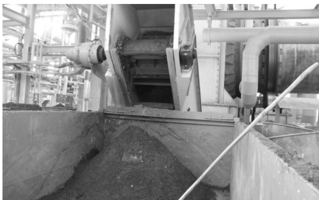
Figure 1. Produced bottom ash (i.e., dumped without treatment).
