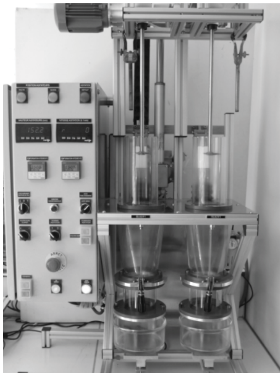
Figure 1. Sludge flocculation device (“boo-test”).
