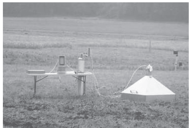
Figure 3. Flux chamber unit installed at field study site.
