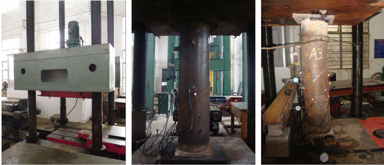
Figure 2. Experiment of the CFST specimens.
