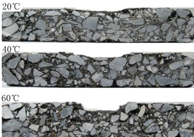
Figure 11. The cross-section graph of rutting at different temperature (AM-40).
