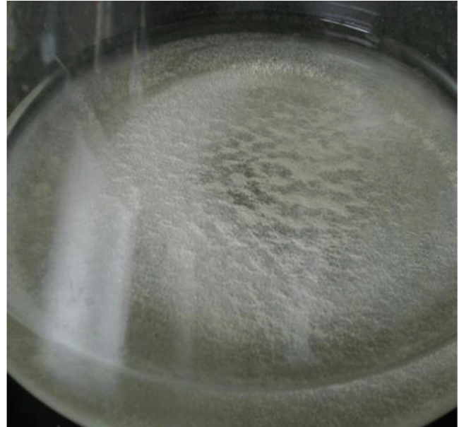
Figure 10. Tail liquid generated by sodium carbonate solution containing 0.8% NT with absorption of hydrogen sulfide.
