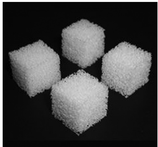
Figure 2. Cubic polyolefin carriers ( 10 \text{ mm} \times 10 \text{ mm} \times 10 \text{ mm} ) used in this equipment.
