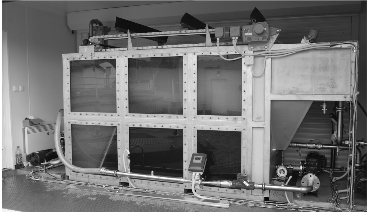
Figure 1. Pilot flotation unit.
