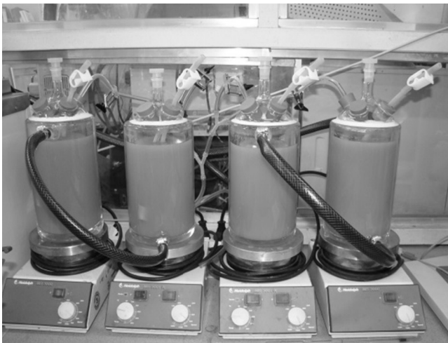
Figure 1. Double-jacket glass tempered cells for denitrification experiments.
