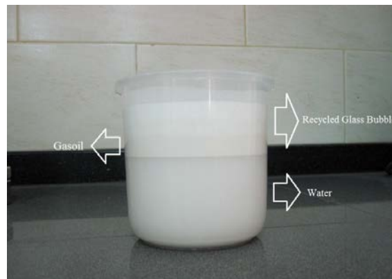
FIGURE 11. THE RECYCLED GLASS BUBBLES BY USING FLOATING METHOD IN THE LABORATORY.
