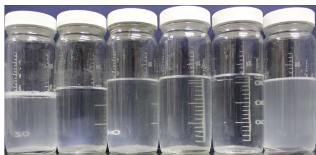
FIGURE 1. BRINE COMPATIBILITY TEST RESULTS FOR DIFFERENT SURFACTANTS AFTER ONE WEEK IN 15% AND 30% BRINES.
