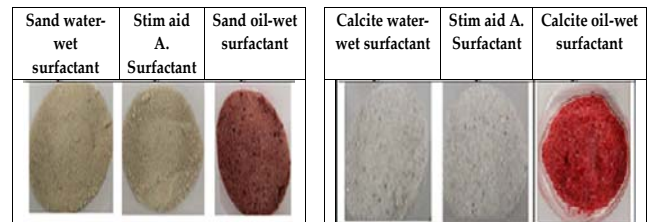
FIGURE 5. WETTABILITY RESULTS IN 15% SYNTHETIC BRINE WITH 40/60 WHITE SAND (LEFT) AND CALCITE (RIGHT).
