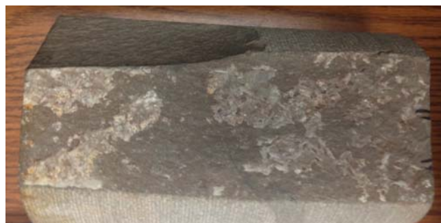
FIG. 19 OBSERVED MINERALIZATION ON FRACTURE SURFACE FROM SPRABERRY CORE
