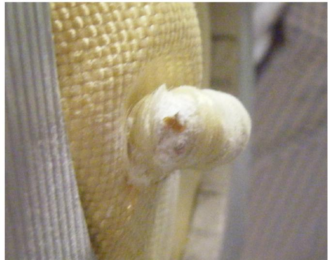
**Figure 10.** Illustration of the importance of the friction between the pulverized Crushmat® material and the spheres—Increased yarn pull-out and retention effect on the projectile.
