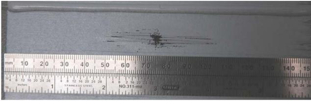
**Figure 8.** Bottom surface of specimen 5-16 after impact at the intermediate energy (8.67 J).
