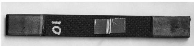
**Figure 3.** Tensile capacitance specimen.
