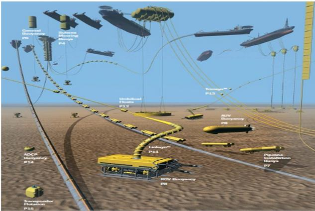
Figure 1. Several products made from syntactic foams [1].
