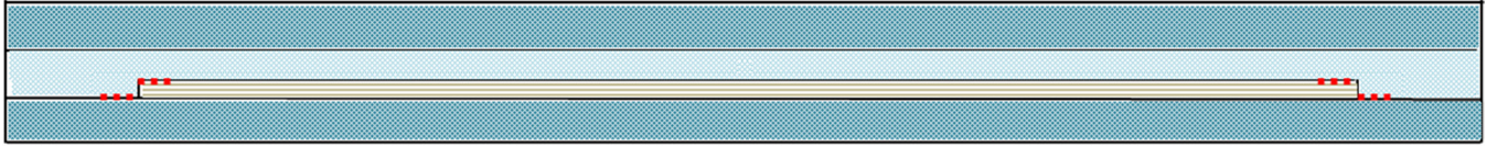
Figure 7. Cross-sectional schematic of the TFB with locations of disbanded areas, as shown in Figure 6, highlighted with dotted lines.
