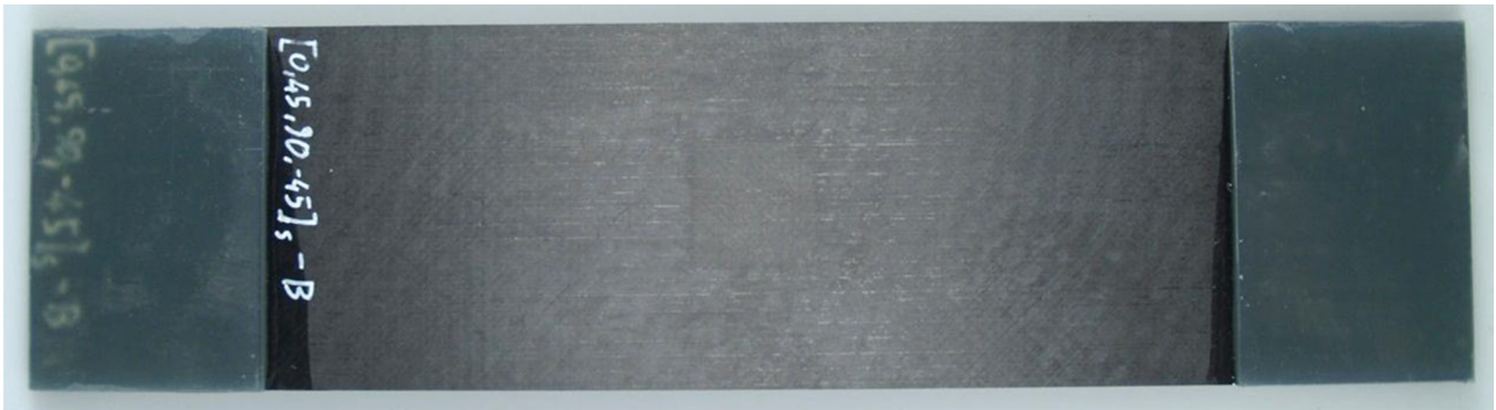
Figure 8. Uniaxial mechanical tension test specimen with embedded TFB at laminate mid-plane. Laminate stacking sequence is (0/45/90/-45/TFB/-45/90/45/0).
