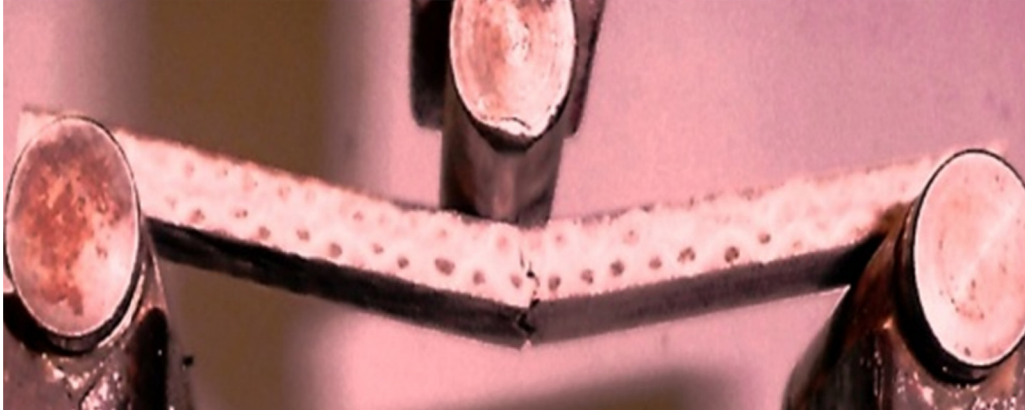
Figure 2. Flexural test setup of composite specimen.
