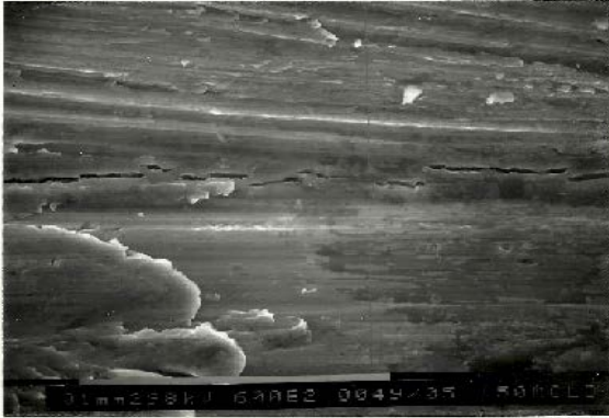
Figure 5 Microcracks initiation at 10 cycles
