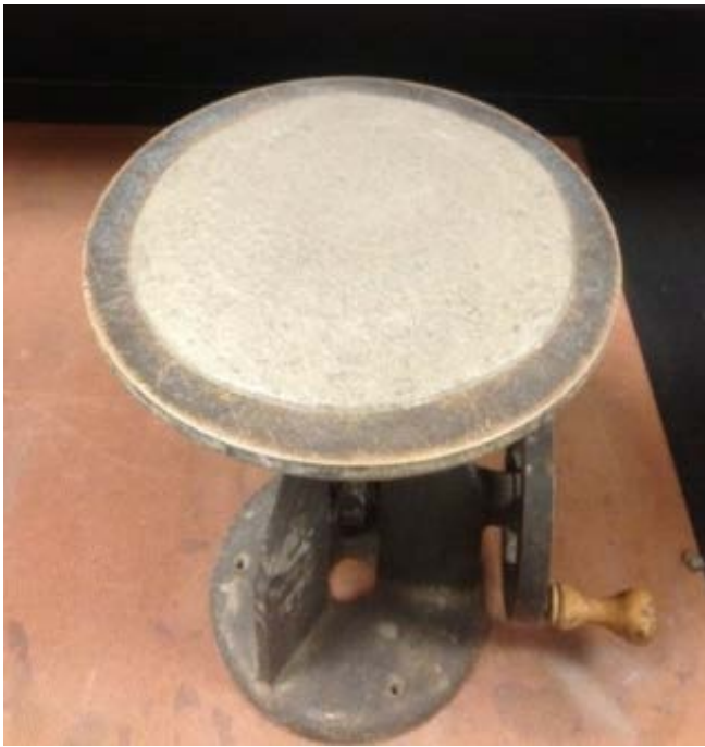
FIGURE 4: FLOW OF MORTAR AFTER THE DROP
