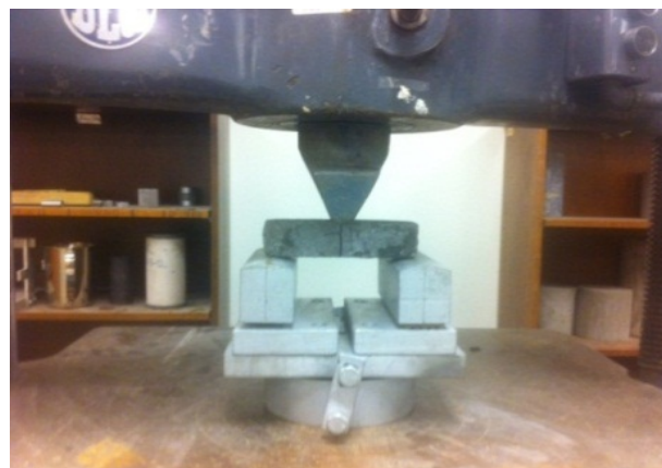
FIGURE 3: FLEXURAL STRENGTH TEST SET UP
