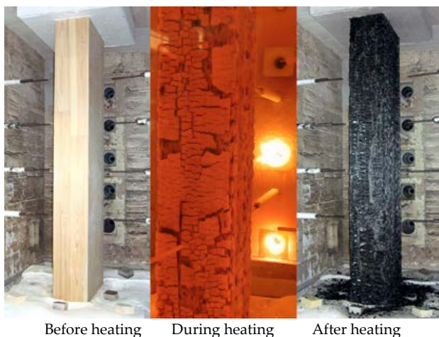
FIG. 5 FIRE TEST OF GLULAM.
