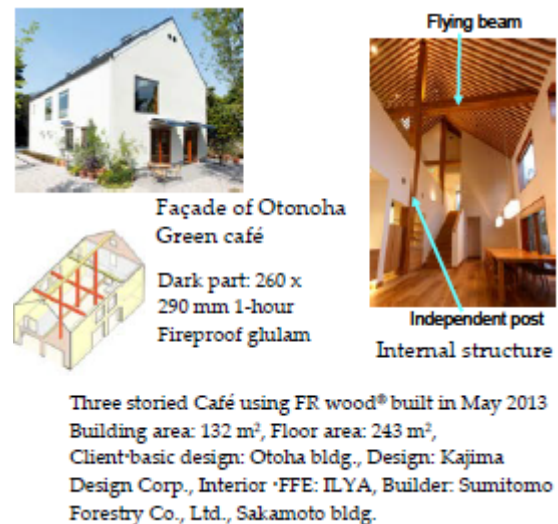
FIG. 7 STRUCTURE OF FIRE-PROOF GLULAM DEVELOPED.
