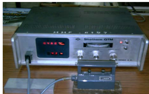
FIG. 4 PICTURE OF THE SHOTHERM-QTM TEMPERATURE MEASUREMENT GAUGE
