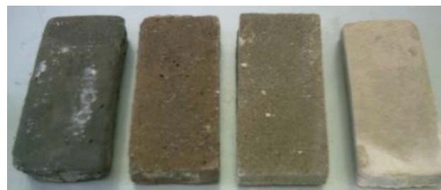
FIG. 3 SAMPLES CONTAINING EVO [EZO (50%), EPO (50%), ESFO (50%), ESO (50%)], FA (50%) AND C (50%), AFTER FIRING
