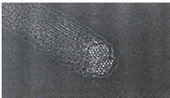
FIG.2 HIGH RESOLUTION ELECTRON MICROSCOPY IMAGE OF SWCNT BUNDLE AS NANOCANTILEVER CLAMPED-FREE DESIGN
