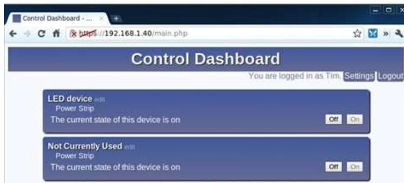
FIGURE 3. CONTROL DASHBOARD –MAIN SCREEN
