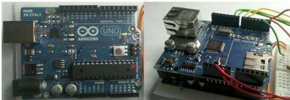
FIGURE 9. ARDUINO BOARD (LEFT) AND AN ETHERNET SHIELD TACKED ON TOP OF AN ARDUINO BOARD (RIGHT)
