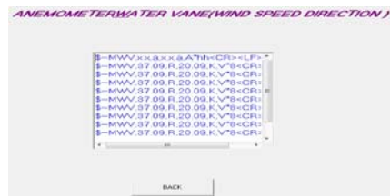
FIG. 19 WIND SPEED DIRECTION SENSOR DATA RECORDED
