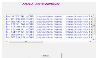
FIG. 15 HULL OPENINGS SENSOR DATA RECORDED
