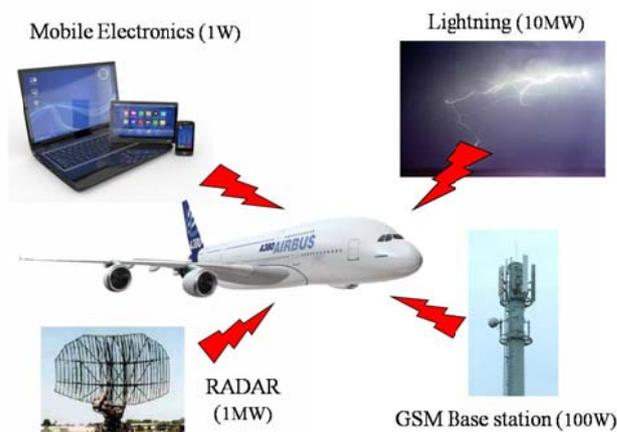
FIG. 1 EXAMPLES OF ELECTROMAGNETIC DISTURBANCES FOR A PLANE
