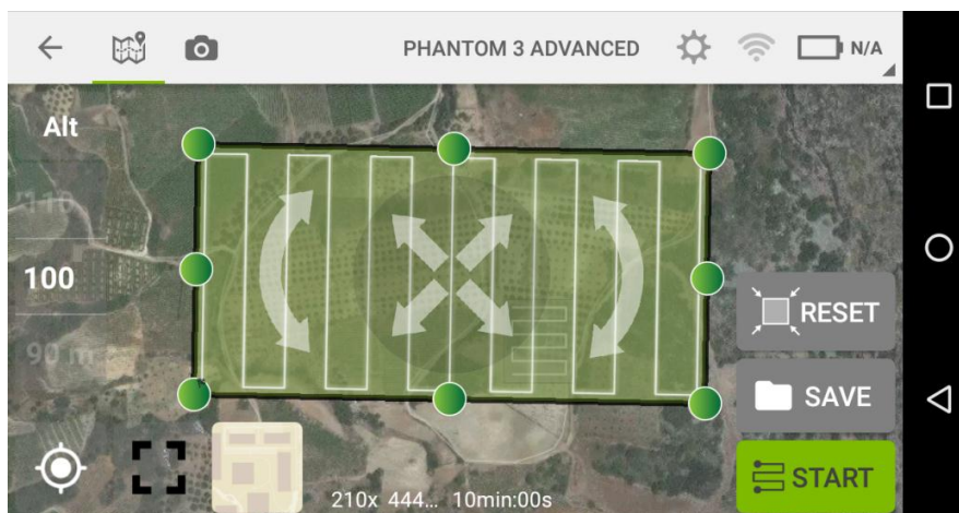
FIG.1 MISSION PLANNING APPLICATION EXAMPLE(PIX4DCAPTURE)
