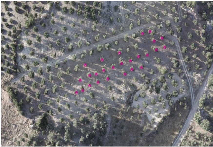
FIG.6 HIGH RESOLUTION GEO-REFERENCED IMAGE(TRUE ORTHOMOSAIC)SHOWING THE 26 OLIVES TREES THAT HAD DRIED FOLIAGE
