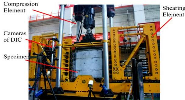
FIG.3 EXPERIMENT SETUP OF STIFFENED COMPOSITE PANELS
