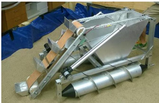
FIG. 1 WURMC'S SCREW-PROPELLED AUTOMATED REGOLITH COLLECTOR
