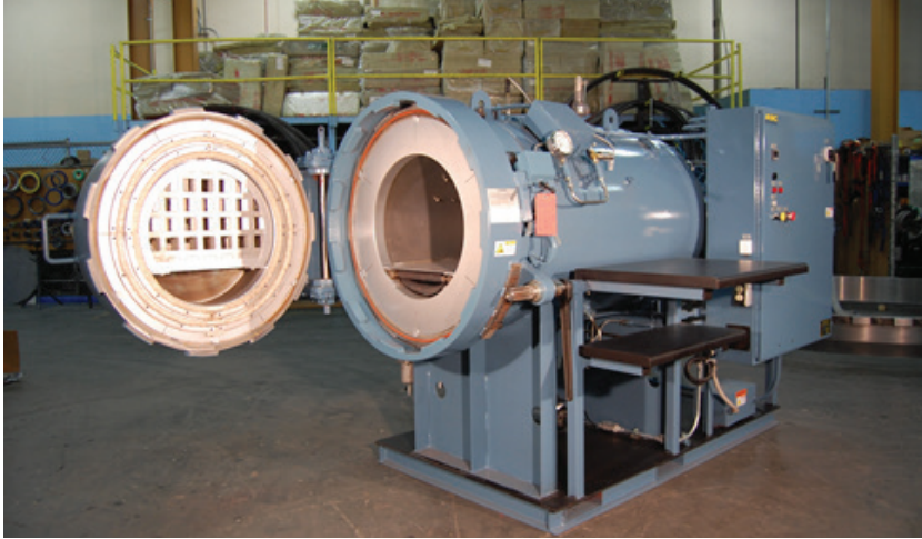
FIGURE 1.1c Photograph of an autoclave.
