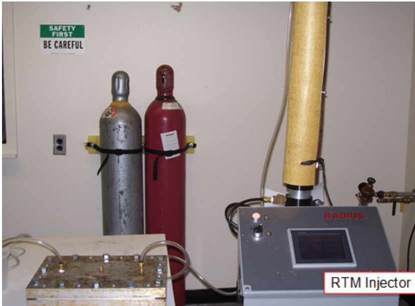
FIGURE 1.4c Instrumentation for liquid composite molding: Pump, mold, and accessories. Resin is filled into the vertical cylinder and then pumped into the mold cavity on the left-hand side.
