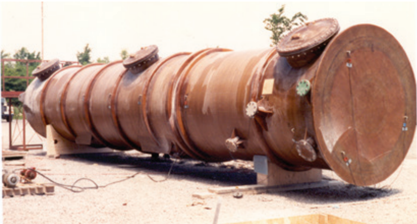
FIGURE 1.2a Composite pressure vessel made by combination of hand-lay-up and filament winding.
