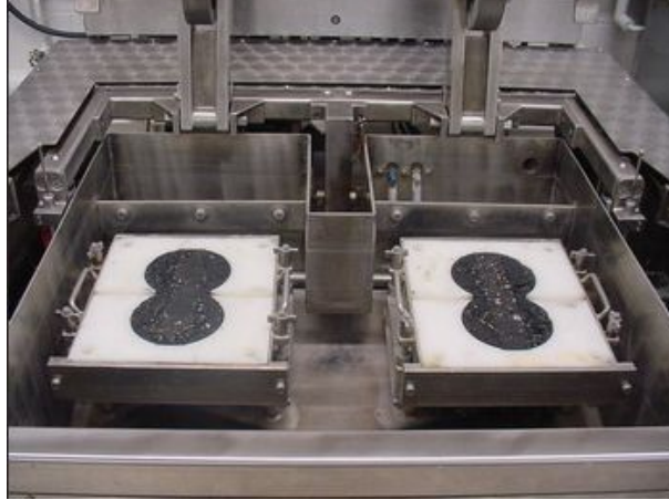
Figure 2. HWTT test equipment.
