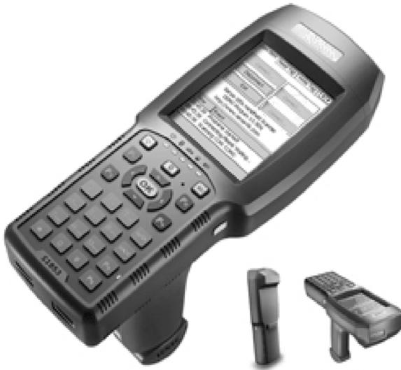
FIGURE 21.2. Portable UHF Reader.
