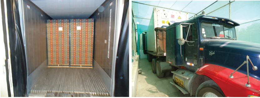
FIGURE 1.19. Palletized loads inside a pre-cooled ISO intermodal container.
