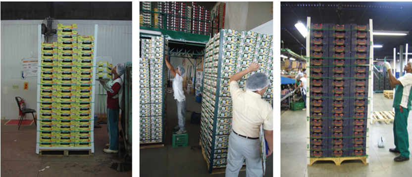
FIGURE 1.18. Palletizing of trays and use of plastic bands to secure loaded pallets.
