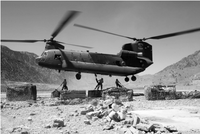
FIGURE 1.2. Deliveries of critical supplies to forward operations by helicopter sling load.
