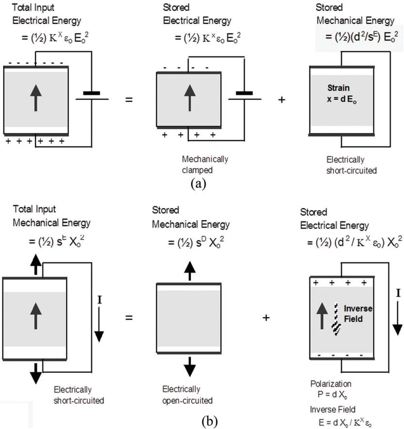
FIGURE 6. Schematic representation of the response of a piezoelectric material under (a) constant applied electric field and (b) constant applied stress conditions.
