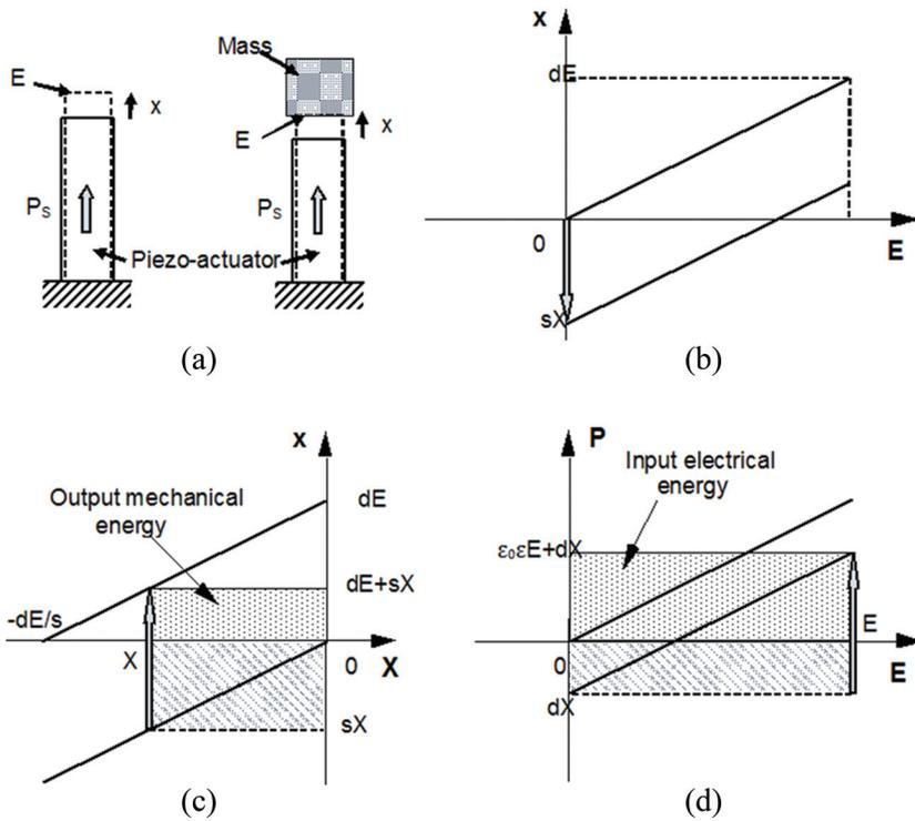
FIGURE 4. Calculation of the input electrical and output mechanical energy: (a) load mass model for the calculation; (b) electric field versus induced strain curve; (c) stress versus strain curve; and (d) electric field versus polarization curve.
