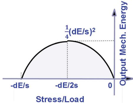
FIGURE 5. Calculation of the maximum output energy.
