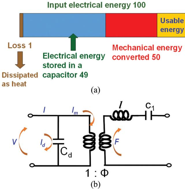
FIGURE 3. (a) Energy conversion rate in a typical piezoelectric. (b) Equivalent circuit ( $k_{31}$  mode).
