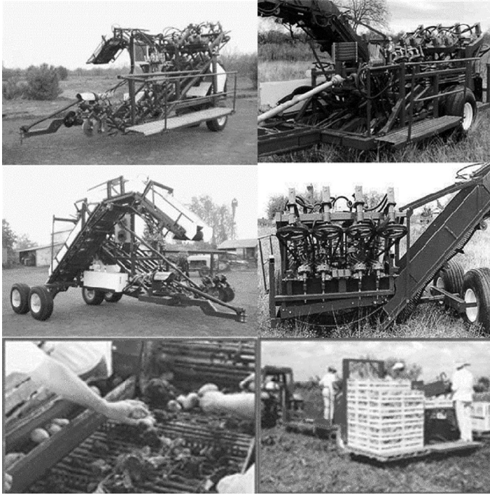
FIGURE 5.5. Diggers for carrots and potatoes.
