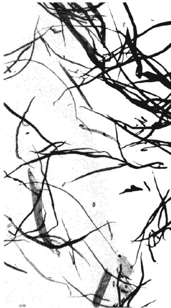
FIGURE 6.3. Shorter stiffer hardwood pulp fibers. Reprinted with permission of TAPPI, from Parham and Gray, Practical Identification of Wood Pulp Fibers (1982), iii.
