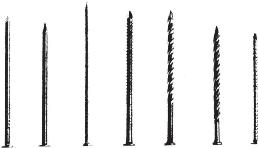
FIGURE 4.1. Various types of nails (left to right); bright smooth wire nail, cement coated, zinc coated, annularly threaded, helically threaded, helically threaded, and barbed (Forest Products Laboratory 2010).
