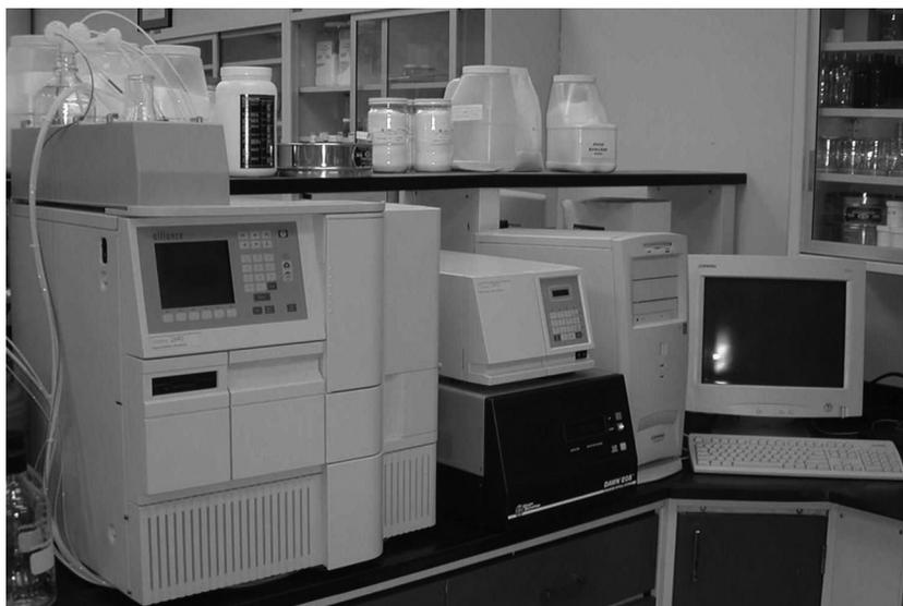
FIGURE 7.2. A Waters HPLC equipped with MALLS and DRI detectors.
