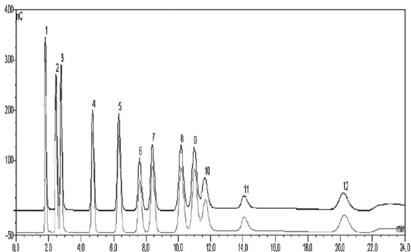
**FIGURE 7.1.** Analysis of the “standard mixture” including 12 carbohydrates and sugar alcohols; concentration = 10 mg.nL for each carbohydrates. Peaks: 1, inositol; 2, sorbitol; 3, mannitol; 4, fucose; 5, salicin; 6, rhamnose; 7, arabinose; 8, galactose; 9, glucose; 10, sucrose; 11, fructose; 12, raffinose. Reprinted with permission from Raessler et al., *J. Agric. Food Chem.*, 56, 7650. Copyright 2008 American Chemical Society.
