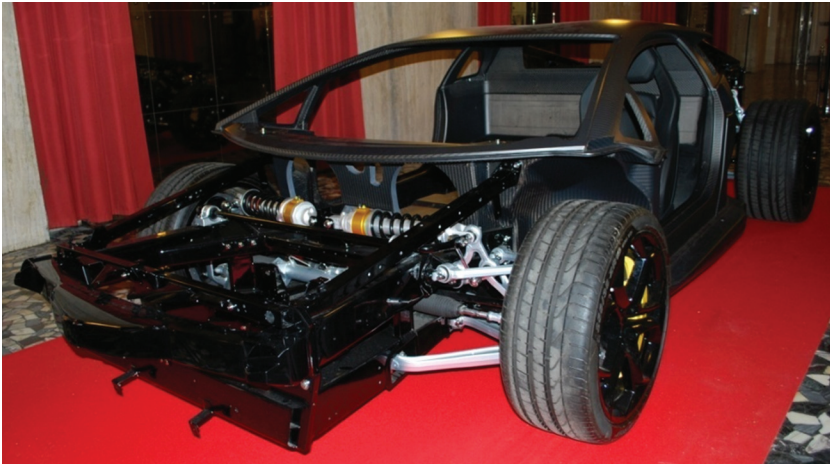
FIGURE 10.3. Chassis of Lamborghini Aventador. Its monocoque forms a single shell in carbon fiber. (Source: Yolanda Ballesteros).
